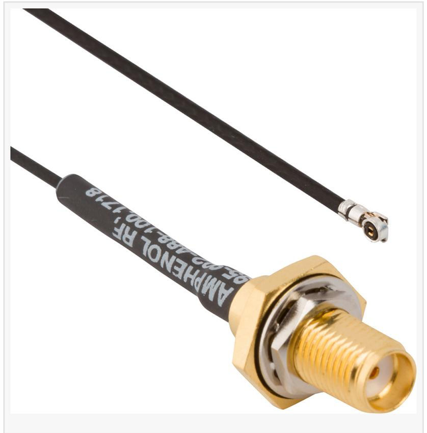
The AMC4 connector is currently the smallest connector in the Amphenol RF portfolio. It shares a similar footprint with the previously released AMMC connector and offers all the same benefits as the AMC interface, but in a more compact package size. This 50 ohm connector offers excellent electrical performance from DC to 6 GHz and is interchangeable with both the I-PEX MHF4 and Murata HSC connectors. The stand-alone version of the AMC4 connector will be available shortly.
