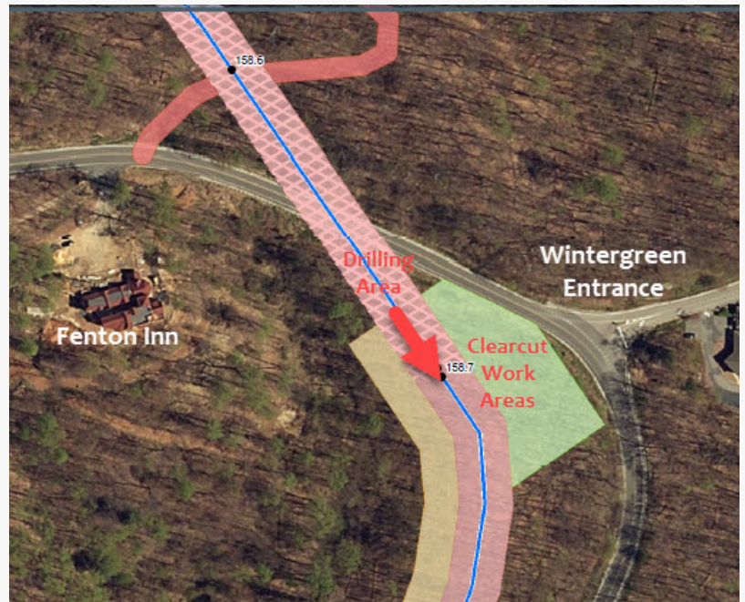
Close up of drilling construction area for 42" pipeline under Blue Ridge Parkway
