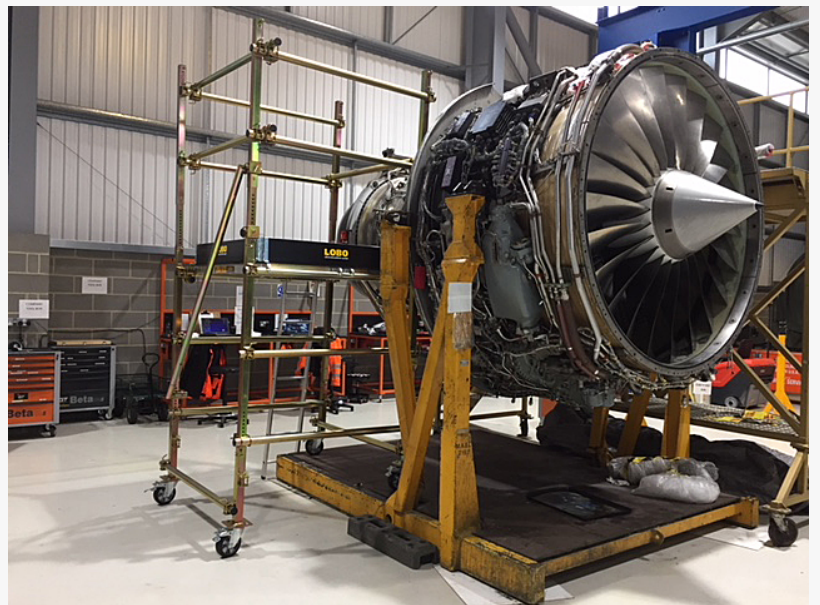
Split level work platform
