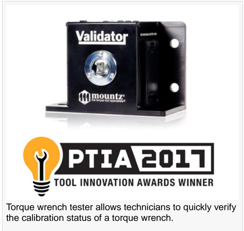
The Validator allows for instant verification that a wrench is still in calibration. Coupled with a torque wrench management and maintenance program the Validator can provide significant cost savings by not relying on a time-based calibration interval but by servicing a wrench only when the wrench starts displaying the incorrect torque during in-house testing.
