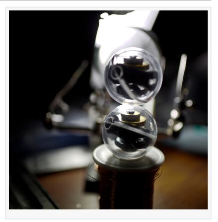
four high-powered Neodymium magnets. The patent pending system features internal gimbals that decouple the motion of the GYRO's surface from its internal magnetic array. This allows the GYROs to move like spherical gears while transparent housings lets you see the mechanism at work.
