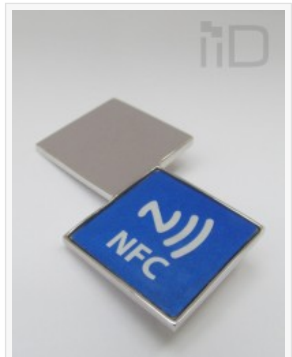
Photo of the first prototype of the iiD, made from Rhodium plated silver with an NFC tag embedded
